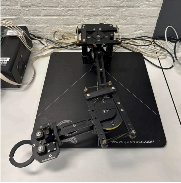
Fig. 2. 2 DoF planar manipulator from Quanser.
