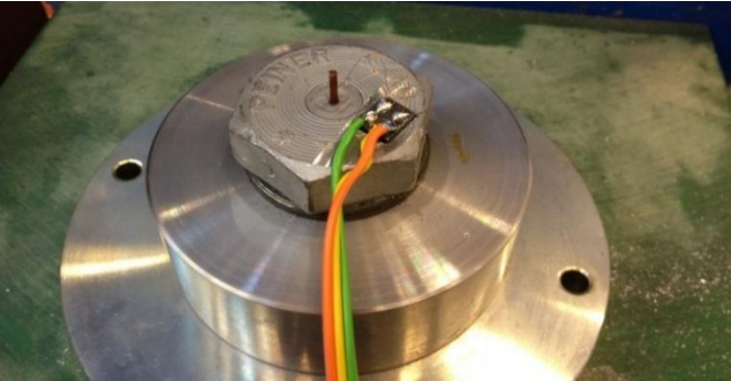
Figure 3.5-1: Hexagonal die used to (1) centre and (2) keep the drill parallel to the bolt axis. Figure 3.5-2: Strain gauge installed in bolt and connected to terminal. Bolt is placed in Skidmore-Wilhelm instrument.
