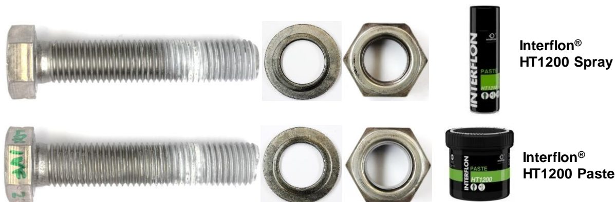
Figure 6.6-5: Bumax – M20x100 bolting assemblies after tightening with Interflon HT1200 spray (above) and Interflon HT1200 paste (below)
