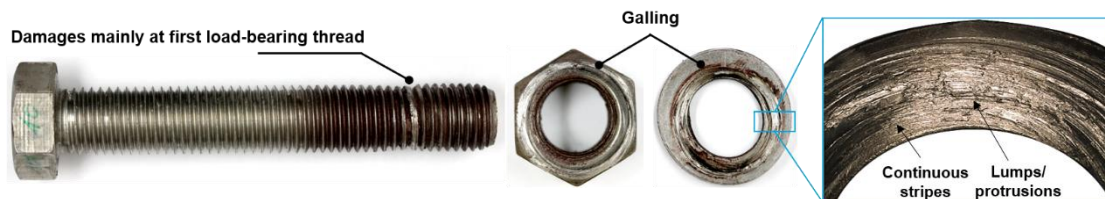
Figure 6.5-2: Galling of the nut bearing surface when tightened into plastic range: bolt (left), nut and washer (middle), and detailed view of washer (right)
