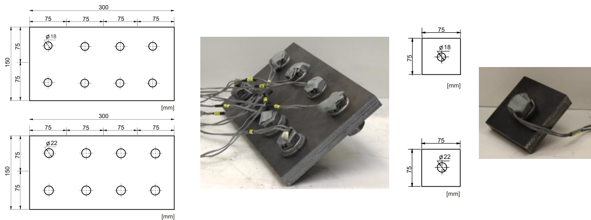
Figure 4.5-4: Test specimen geometry for the relaxation tests of the bolted connections (test specimens for M16 and M20 bolts)
