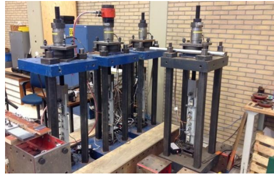
b) test rig for extended creep tests (TUD)
