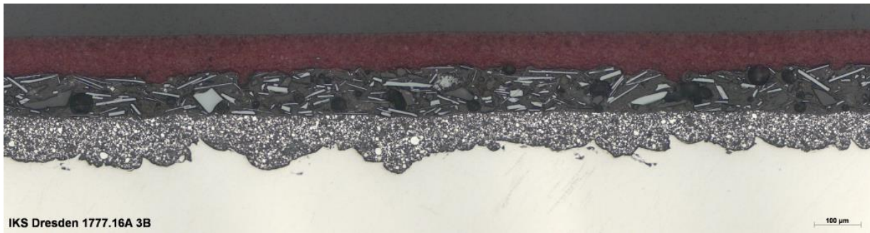
a) Roughness profile of chill casting
