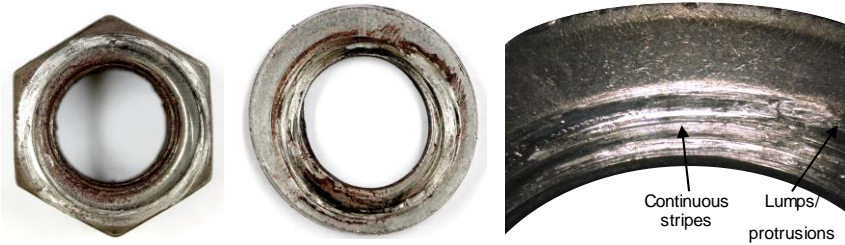
Figure 6.6-2: Galling of the nut bearing surface when tightened into plastic range: nut (left), washer (middle) and detailed view of washer (right)
