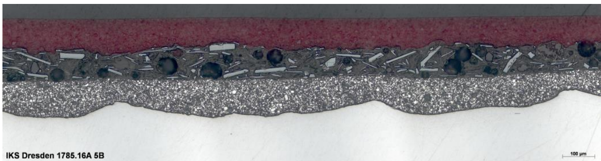
c) Roughness profile of steel casting
