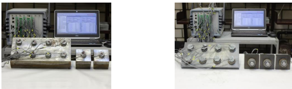
Figure 4.5-5: Exemplary test setup for M16 bolted connection without DTIs (left) and for M20 bolted connection with DTIs (right)
