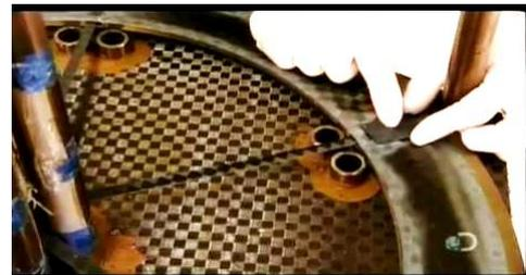
Figure 6.18: A carbon fiber patch is applied on the spoke and the rim side wall [33].
