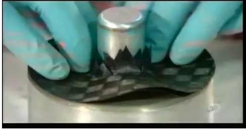
Figure 6.19: Lay-up of the hub using a shaft mold. Flanges cut in the fabric cover the corners [33].
