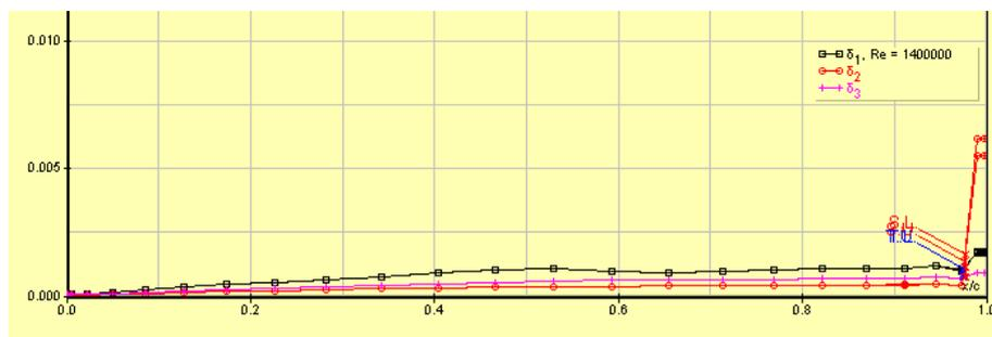
Figure 3.10: The boundary layer analysis of airfoil RU-21T-00632D by Javafoil
