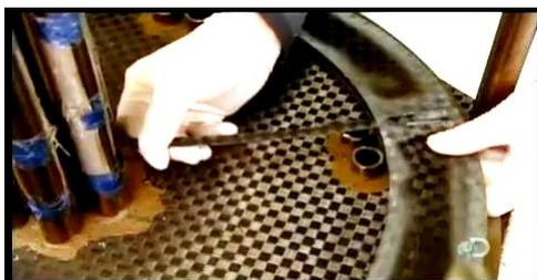
Figure 6.17: Flat spokes are inserted in a small incision in the rim side wall [33].
