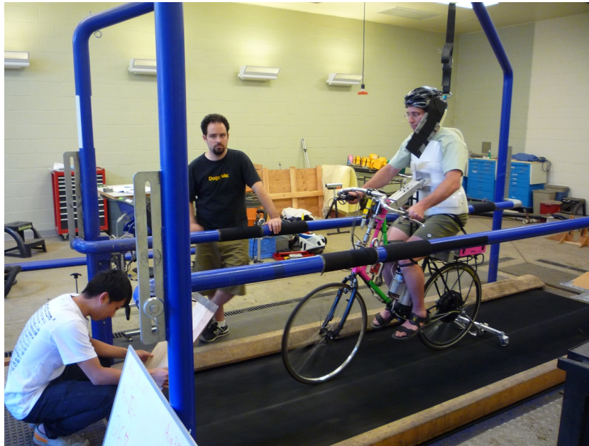
Figure 4.2: A participant of the UC Davis study riding the instrumented bicycle on a horse treadmill (source: [63]).
