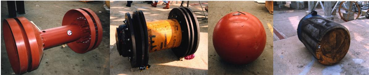
Figure 1.2: Four common pig types: cup pig, bidi pig, spherical pig and foam pig [15].
