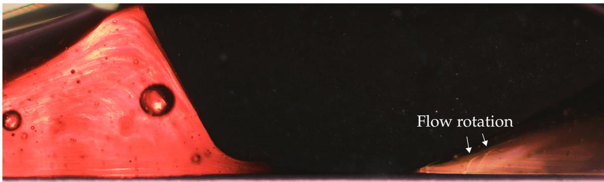
Figure 4.14: Rubber contact during the experimental run with castor oil after the sliding motion has stopped.
