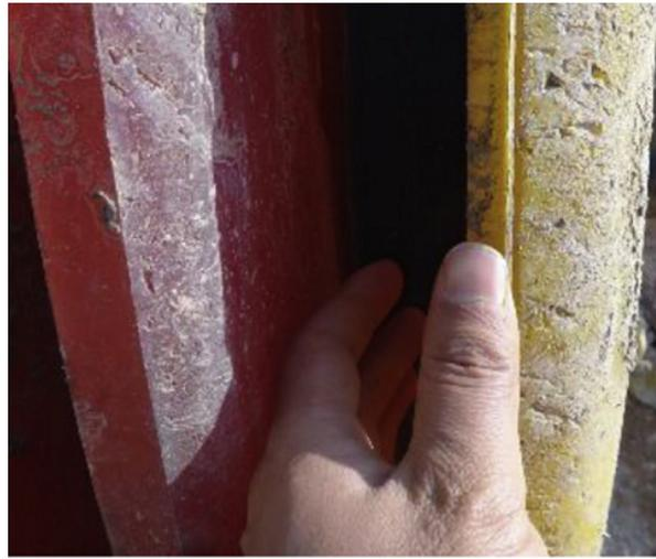
Figure 2.14: Worn sealing and guiding discs of a pig [32].
