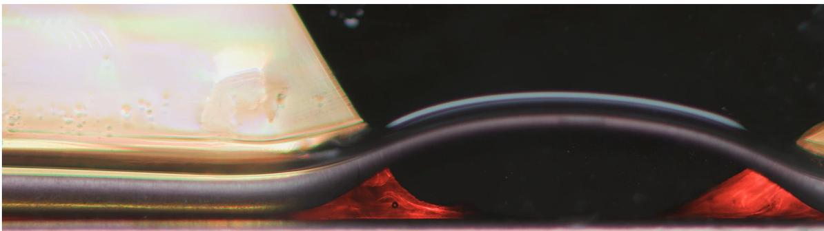
Figure 4.9: Rubber contact during the experimental run with castor oil at a sliding distance of 0 mm.
