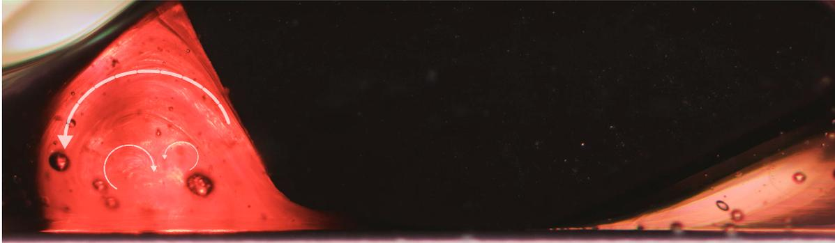
Figure 4.13: Rubber contact during the experimental run with castor oil at a sliding distance of 98 mm.
