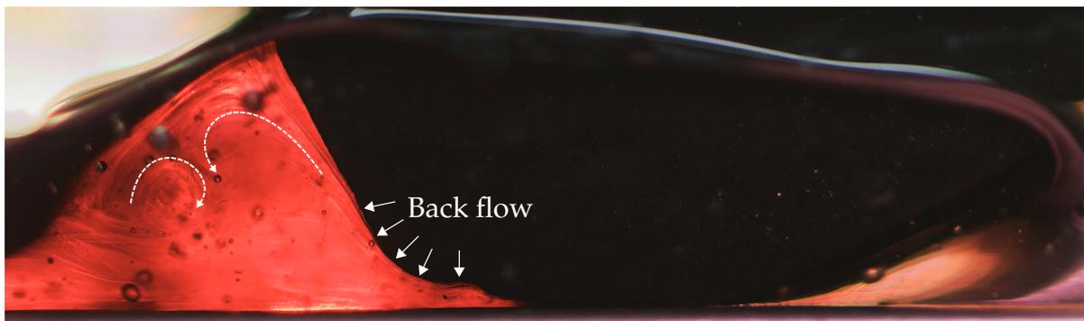
Figure 4.12: Rubber contact during the experimental run with castor oil at a sliding distance of 69 mm.
