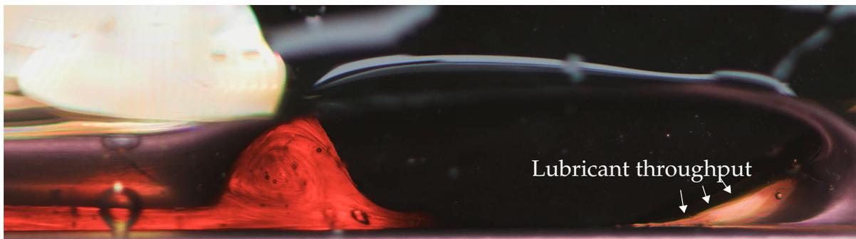
Figure 4.11: Rubber contact during the experimental run with castor oil at a sliding distance of 51 mm.
