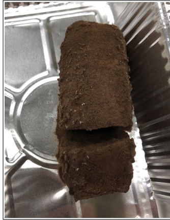
Figure 7.1: Horizontal fracture at 1/3 of the samples height. Retrieved from sample CU10-2.
