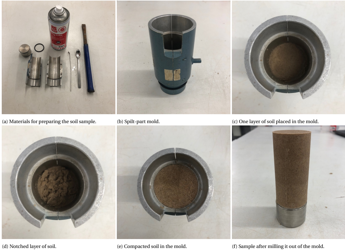
Figure 5.3: Visualisation of the different steps of the sample preparation for the triaxial tests.
