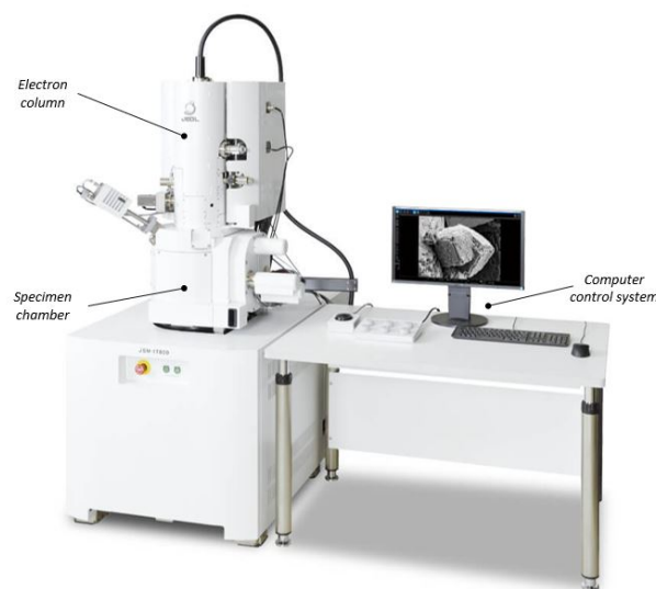
Figure 5.7: The SEM setup showing the three major sections of the SEM: the electron column, specimen chamber and computer control system (Jeol, 2023).
