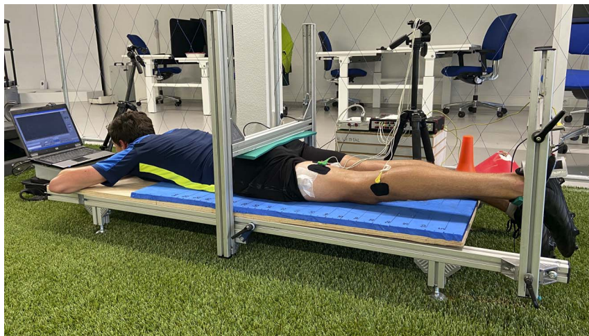
FIGURE 2—Custom build adjustable rigid dynamometer.
