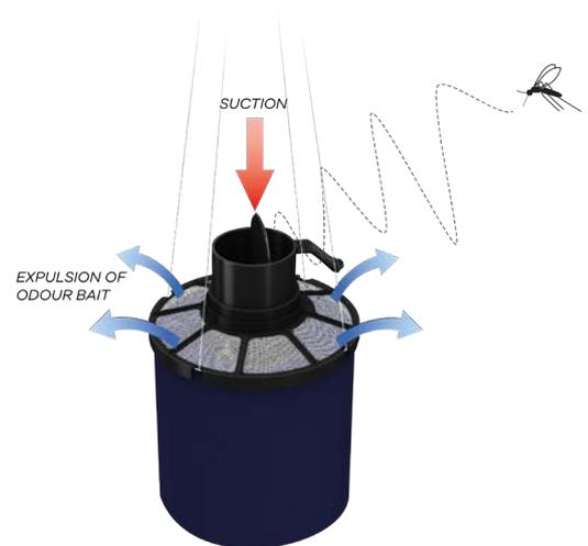
FIGURE 5: SCHEMATIC DRAWING OF COUNTERFLOW TECHNOLOGY
