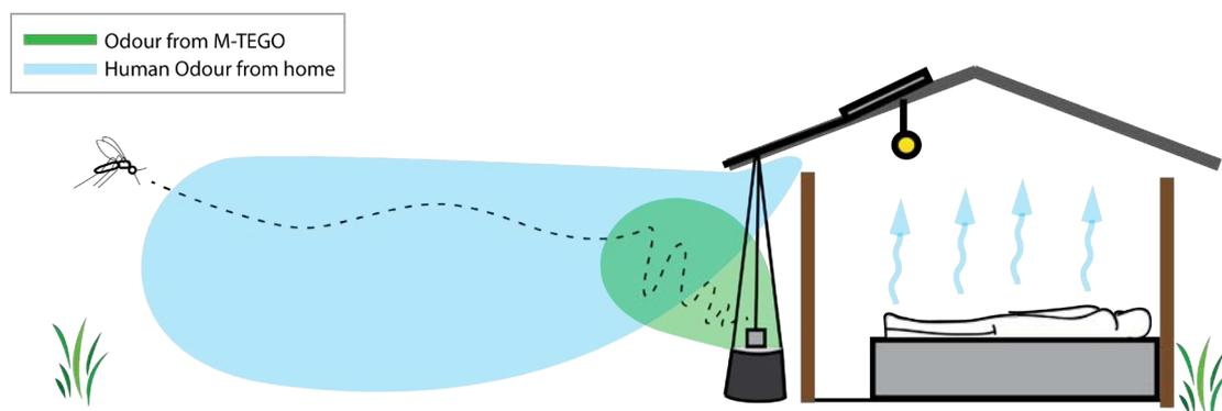
FIGURE 6: SCHEMATIC DRAWING OF MTEGO PRINCIPLE
