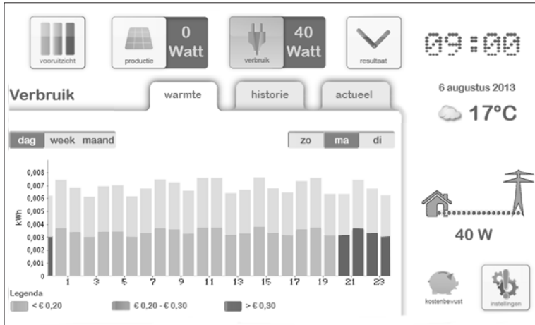
ELECTRICITY USE OF THE HEAT PUMP COMPARED TO THE TOTAL ELECTRICITY USE WITH INDICATION OF FAVOURABLE MOMENTS
