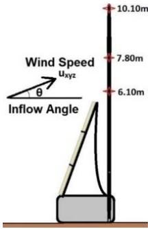
Figure 2 - 10 : Wind speed U_{xyz}(m/s) magnitude vector and the inflow angle \theta ( ^{\circ} ), illustrated for a perpendicular flow indicating the presence of sonic anemometers with red stars in different heights for Pole 1
