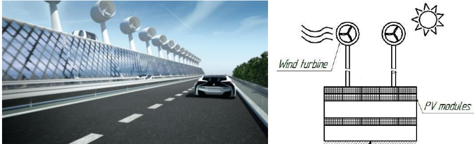
Figure 4 - 11: Illustrations of a combined wind and solar photovoltaic noise barrier
