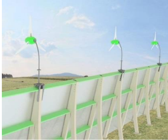
Figure 2 - 1: Visualization of micro wind turbines integrated on a noise barrier
