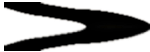
Fig. 14. Cantilever problem optimized using the volume constraint formulation with continuation on q , \frac{C}{C_{ref}} = 130.5\% , V_t = 50\% , 146 iterations.
