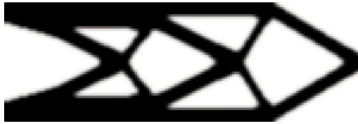
Fig. 8. Free form optimized result for cantilever problem with a reference compliance of \frac{c}{c_{ref}} = 100\% , V_i = 50\% and in 167 iterations.
