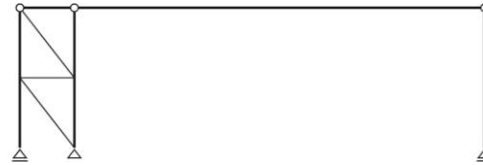
Portal construction (shear connection)
