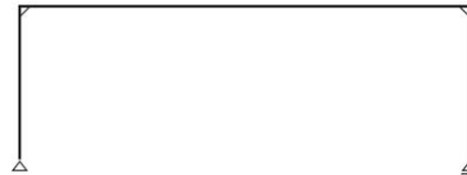
Portal construction (moment connection)
