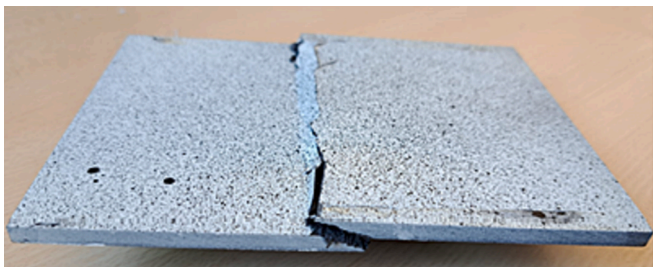
Fig. 4. Failed specimen after the CFAI test.
