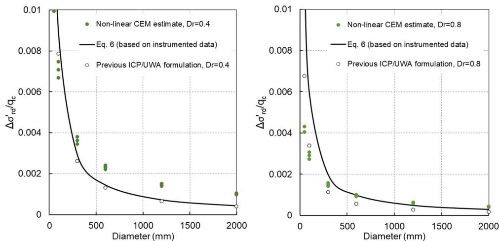
**Fig. 3. Comparison of predictions of  $\Delta\sigma'_{rd}/q_c$  from CE theory with result of regression analysis from instrumented data (Eq. 6) for two relative densities of a sand**
