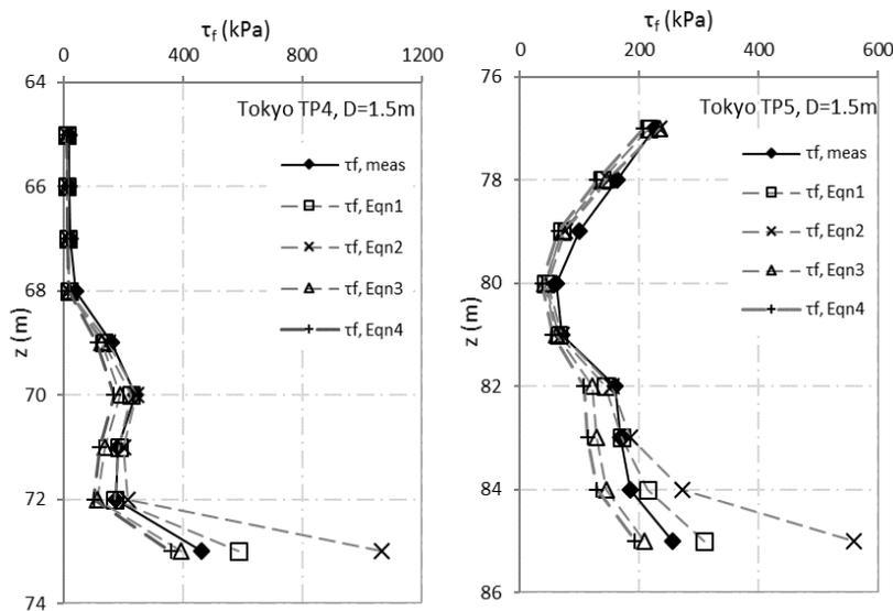
**Fig. 7. Measured and calculated  $\tau_f$  profiles in large diameter piles in Tokyo**
