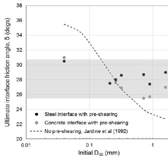
Fig. 4. Variation of interface friction angle with  $D_{50}$
