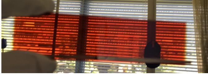
Figure 6.4: Semi-transparent cell sample viewed at the rear with the window as background.
