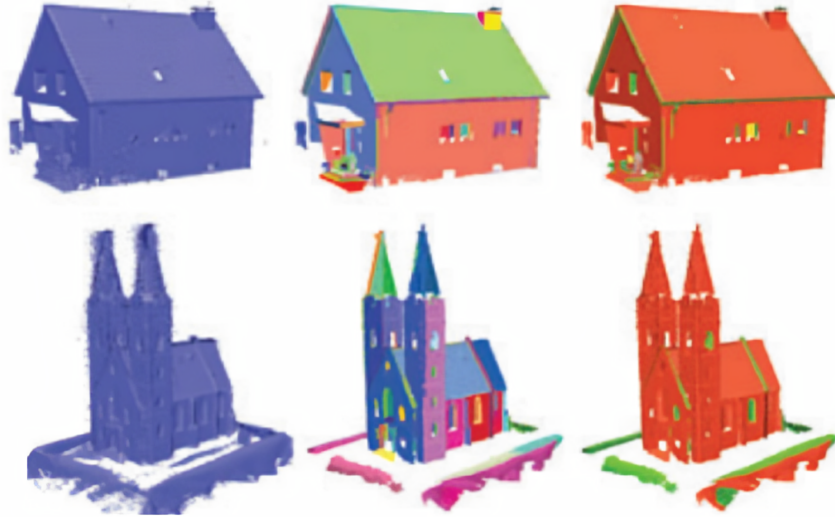
Figure 2.6: Primitives detection with RANSAC. First column: point clouds. Second column: Detected shapes coloured randomly. Last column: Shapes coloured by type [Schnabel et al., 2007].
