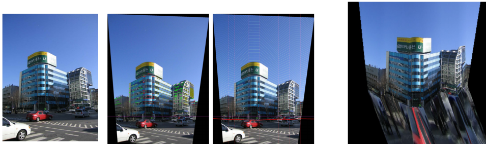
Figure 2.4: Fast automatic single-view 3D reconstruction of urban scenes. From left to right: source image, processed image, different positions of ground-vertical border along the vertical axis, reconstructed scene [Barinova et al., 2008].
