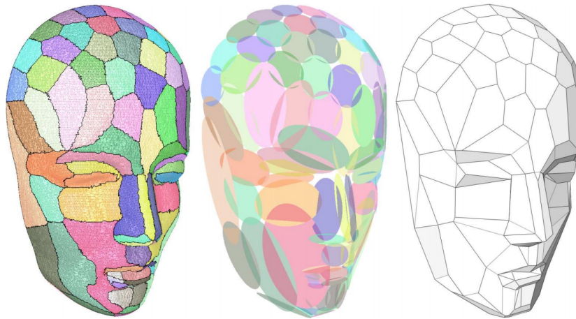
Figure 2.11: Variational shape approximation (VSA). From left to right: error-driven partitioning, geometric proxies and approximated polygonal mesh [Cohen-Steiner et al., 2004].
