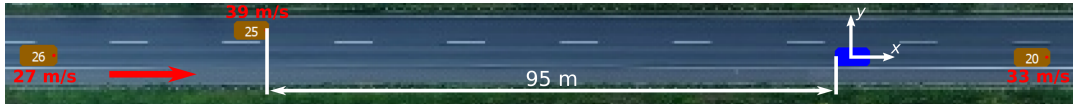
Fig. 3. The hand-picked example of the traffic scene of interest, as it is used in step 1 of our case study (highD dataset 1, frame 379, ego vehicle id 21). The blue vehicle is the ego vehicle, with the red arrow indicating the driving direction. The orange vehicles (id 25,26,20) denote other traffic participants, making up the traffic context, all driving in the same direction on the two-lane highway. In this example, the driver could decide to stay behind the vehicle it is currently following (id 20), but could also decide to accelerate and overtake that vehicle. The white arrows depicting x and y show the ego vehicle's reference frame. The gap between vehicle 25 and the ego vehicle is 95 meters. The numbers in red denote the longitudinal velocities of the surrounding vehicles.
