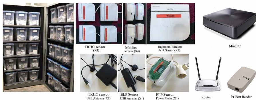
FIG. APP.C.1 The boxes with equipment inside: Each box was sent to one house and the equipment were installed. All the equipment are coded and labeled and coupled with the database.
