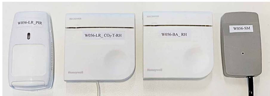
FIG. 6.1 Sensors used in the measurement campaign, from left to right: motion sensors (4 rooms), CO 2 -air temperature-RH sensor (4 rooms), RH sensor (bathroom), and smart meter port reader
