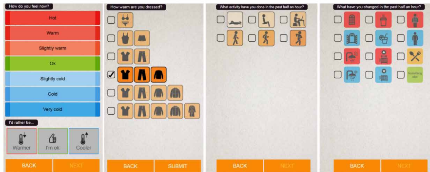
FIG. APP.C.2 An example of the questions asked in the comfort app: The occupants fill the app occasionally and the data is saved in the servers for further comparison and analysis.
