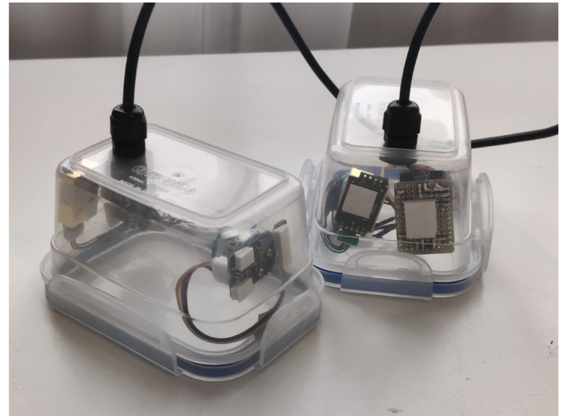
Figure 66. Bioprinted constructs can be placed in these boxes to measure the CO 2 , O 2 and temperature.
