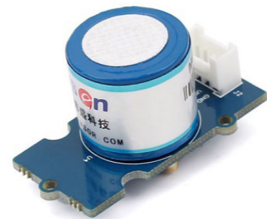
Figure 64. The O 2 sensor used to measure the photosynthetic ability of the bio-ink
