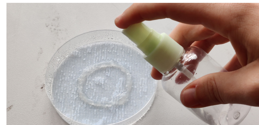
Figure 41. Extruding sodium alginate (5 w/v%) crosslinking it by spraying calcium chloride (5M) each layer.
