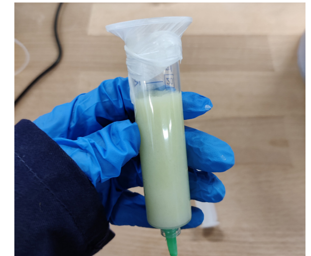
Centrifuging the syringe with bio-ink (step 14)
