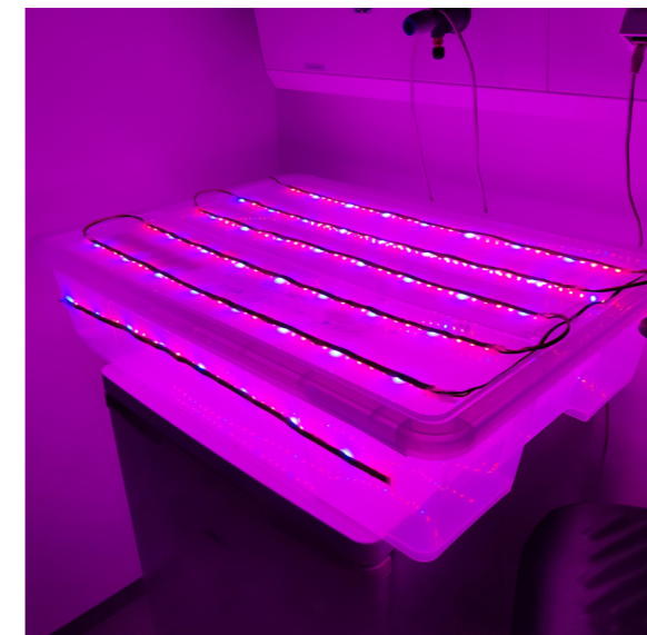
Figure 35. Incubator where microalgae bioprints are placed after they are 3D printed and crosslinked.
