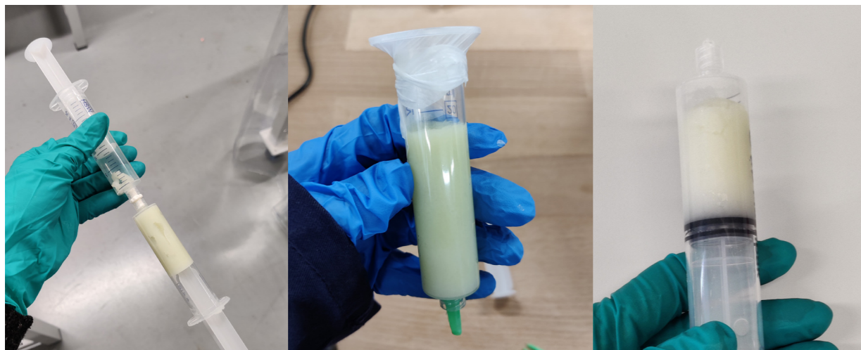
Figure 55. Approaches to remove air bubbles in the syringe barrel. From left to right: Bottom up filling with a coupler, centrifuging and vacuuming.
