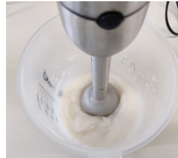
Blend autoclaved ink for two minutes (step 5)
