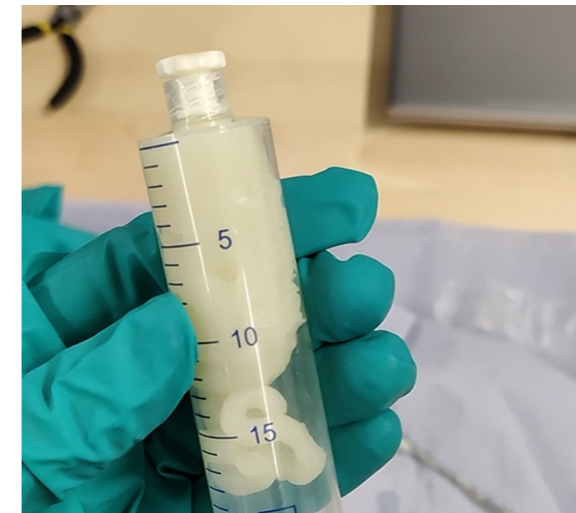
Adding bio-ink to the syringe (step 12)
