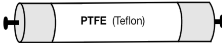
Figure 3.2: Separate parts are assembled by screwing the electrodes into the PTFE insulation.
