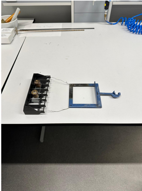
(a) Conventional plough with additional weights
