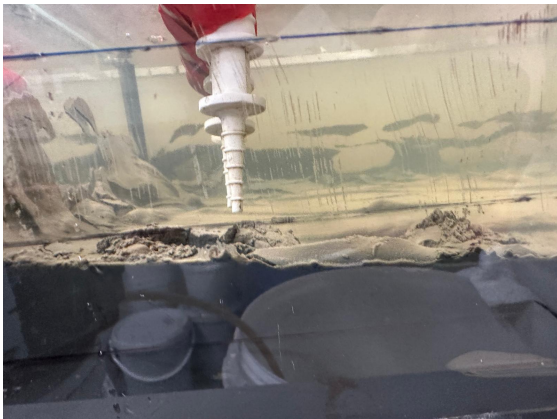
(c) Test setup of submerged WID prototype
