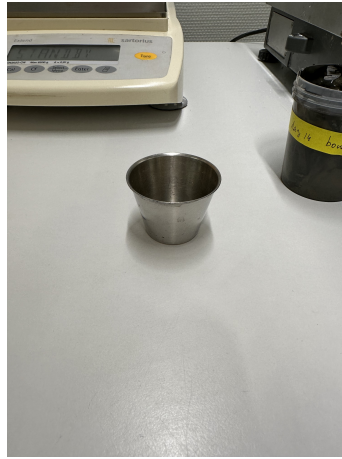
Figure 20: Container for measuring density
