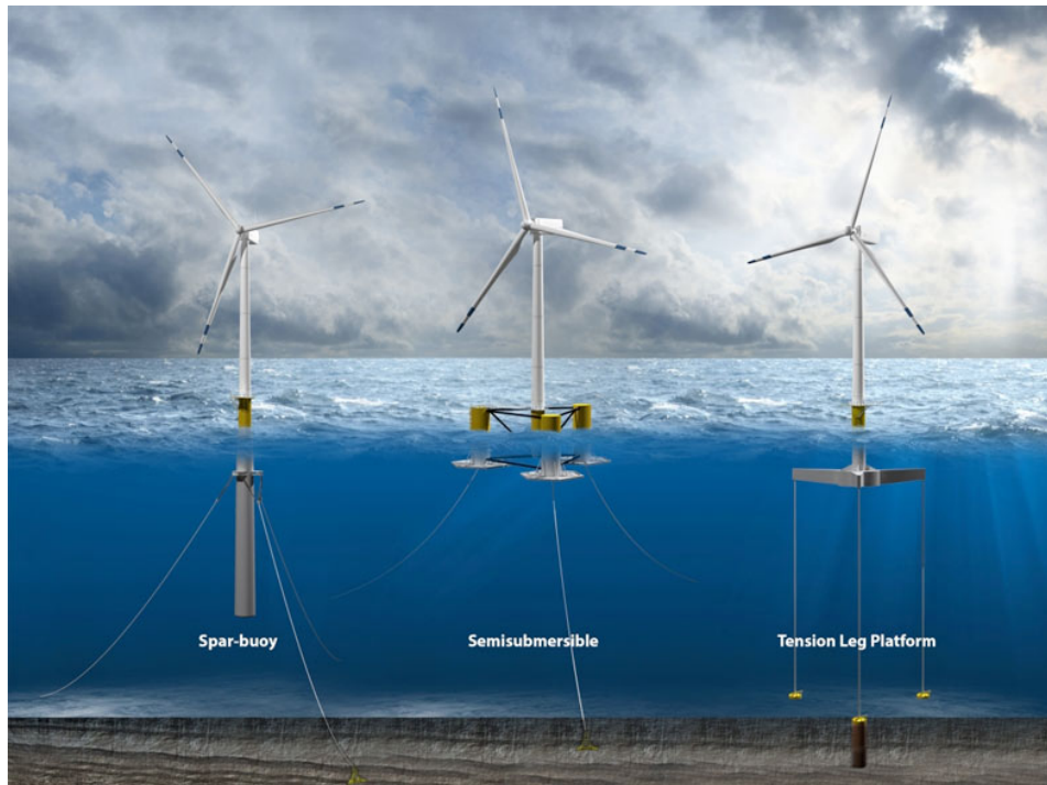
Figure 2.2: Three types of deep sea mooring for offshore wind turbines [92]
