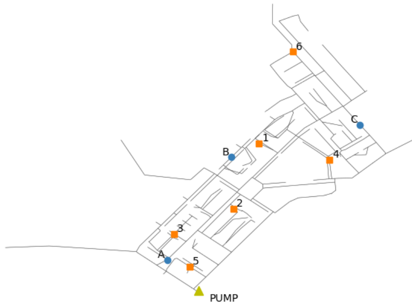
Figure 3.6: Simulated leak (alphabetical letters) and sensor locations (numbered)
