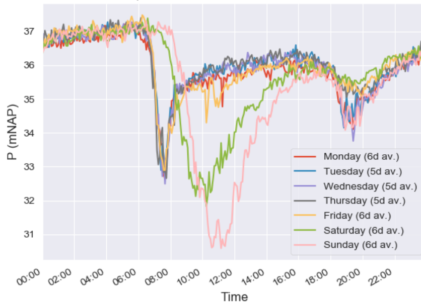
Daily average Pressure at the PUMP for different days in the week in period: 2019-03-08 - 2019-04-16
