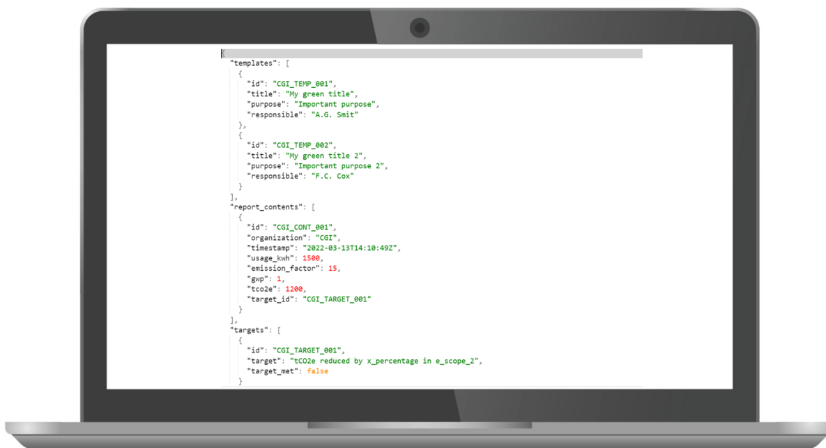
Fig. 27: Illustration of JSON formatted data wherein user receives carbon accounting data from CAS.
