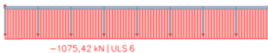
Figure D-18: Normal forces in the beams in the y-direction (for ULS 6)
