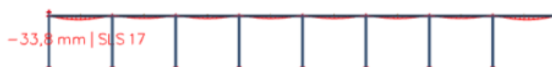
Figure B-18: Vertical deflection for governing characteristic load combination (SLS 17) for the y-direction
