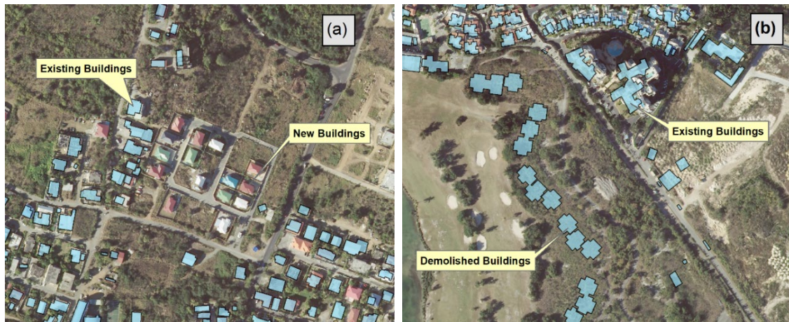
Figure 2.1. Sources of buildings data – OSM, VROMI and SPOT satellite image. (a) Shows the buildings shapefile extracted from OSM using the satellite image as a background. The blue polygons represent buildings existing in the database whereas the rest are new buildings missing in the OSM database. (b) Shows the VROMI shapefile in beige and red line over the SPOT image. It is observed that some buildings have been demolished.
