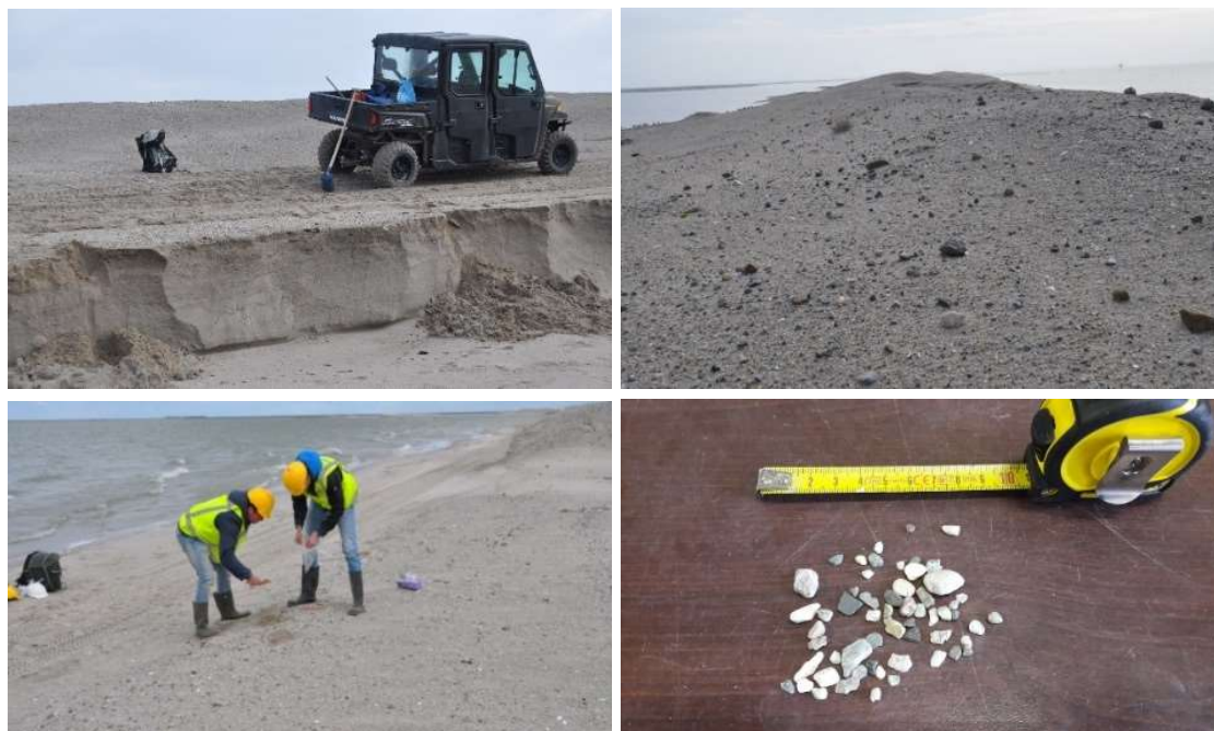
Fig. 3. Field trip to the Marker Wadden. Top left: Beach scarp formation along the sandy ridge. Top right: Desert pavement development on top of the artificial dune. Bottom left: Sediment sampling from the subaerial domain. Bottom right: Remaining sediment fraction after sieving a sediment sample from the desert pavement (photographs by B. van der Valk).
