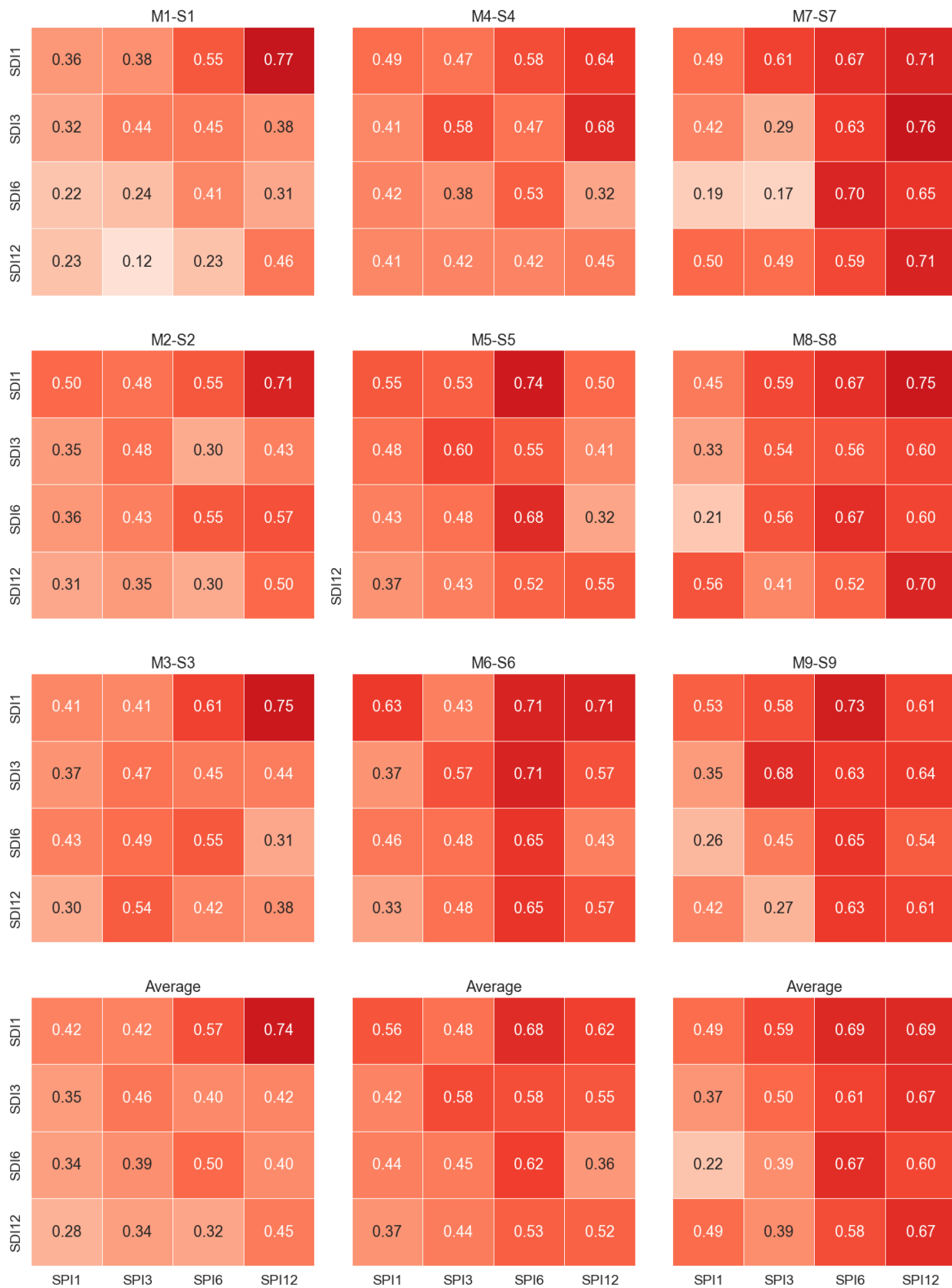
FIGURE 7 Formative drought rate (FDR) matrix of propagation from meteorological drought in SPI_k to hydrological drought in SDI_m for station pairs ( k = 1, 3, 6, 12 months; m = 1, 3, 6, 12 months). Matrices in the upper three lines of the figure show the FDR associated with each cell calculated as the average of each station pair. Matrices in the lower line show the average of river basins. Darker shades in the cells indicate higher values of FDR.
