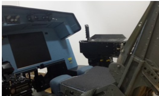
Figure 5-5: Fixed-base simulator setup in the Human-Machine Interaction Laboratory with the sidestick installed on the right side of the pilot seat.
