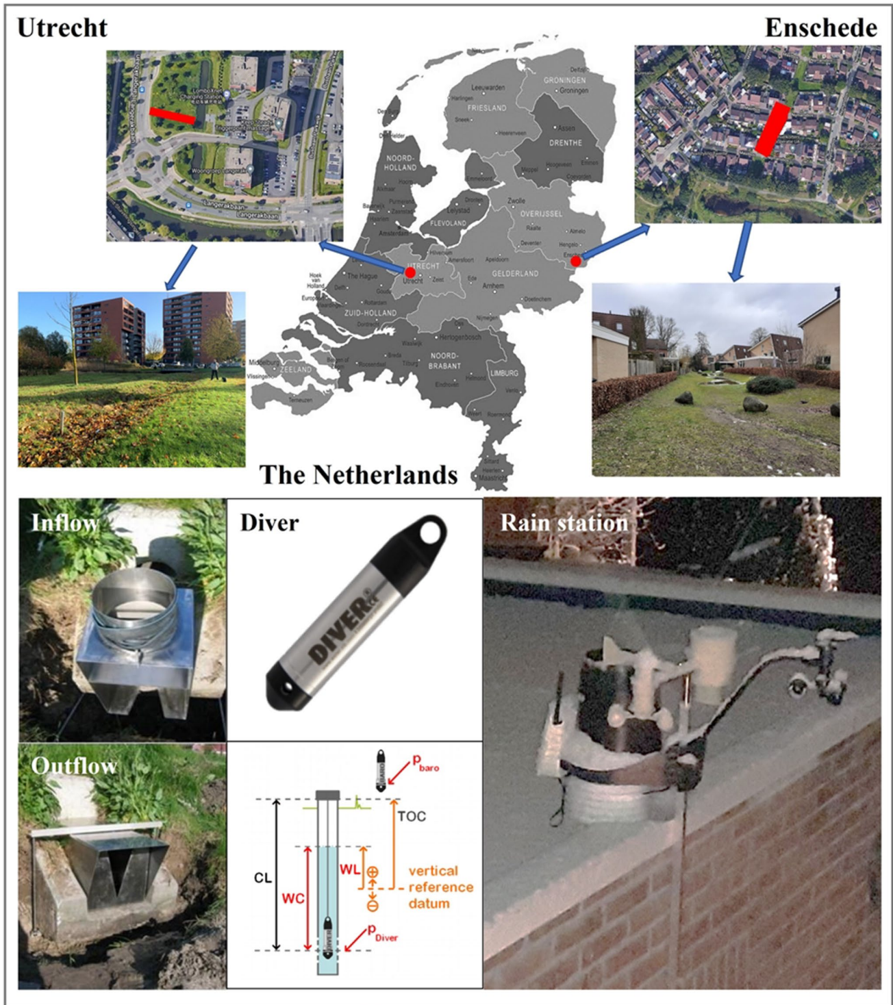
Fig. 1 Location and monitoring equipment of two target grassed swales in the Netherlands
