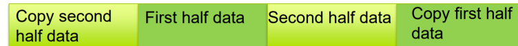
Figure 4.3: Aliasing trick. A copy of the second half of the data is placed in front of the first half of the data and a copy of the first half of the data is placed after the second half of the data.
