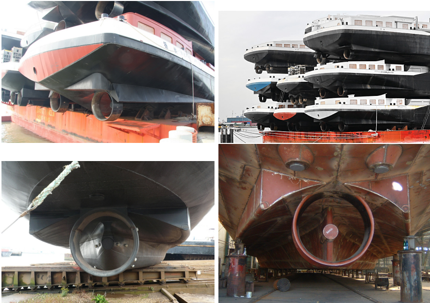
Figure 3.4: Inland ships on pontoons during transport. One aspects to be observed between the sterns is that the distance between the propeller ducts differs among the ships (photos by René Rapati, Groenendijk & Soetermeer)
