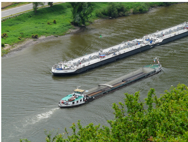
Figure 2.1: An inland ship sailing with small freeboard
