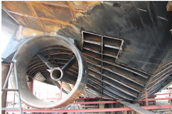
Figure 3.5: The tunnel of an double propeller inland ship under construction. The tunnel frames can be identified and by taking the highest point in each frame, one can draw the tunnel top curve and see that for this specific ship, the tunnel is such that the flow enters the duct and propeller under an angle. (photo by René Rapati, Groenendijk & Soetermeer)
