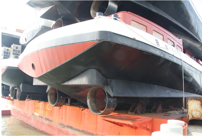
Figure 1.4: Stern of an inland ship on a transport barge, showing propeller ducts and tunnel skirts. The ship in the foreground features a headbox as well. Headboxes, however, are not studied in this thesis. (Photo by René Rapati, Groenendijk & Soetermeer)
