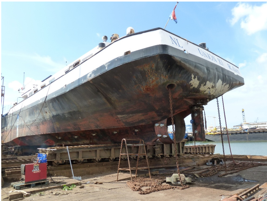
Figure 2.4: Example of an inland ship stern with a tunnel, but integrated tunnel skirts (Photo by René Rapati, Groenendijk & Soetermeer)
