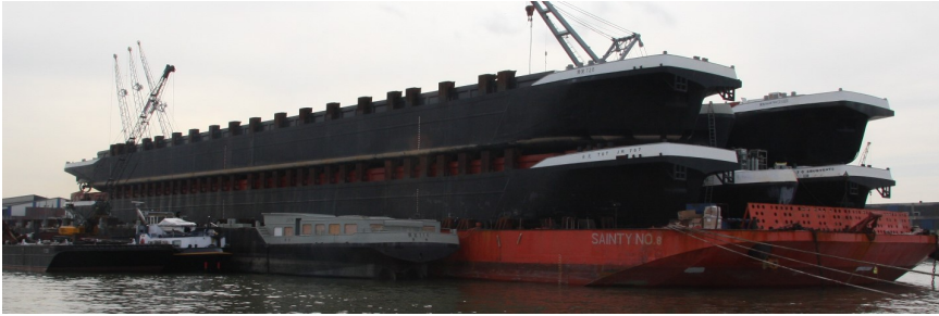
Figure 2.2: Inland ships with a length of 135.0 meters stacked on a pontoon. The long parallel midship, and the short bow and stern regions, are visible. (Photo by René Rapati, Groenendijk & Soetermeer)
