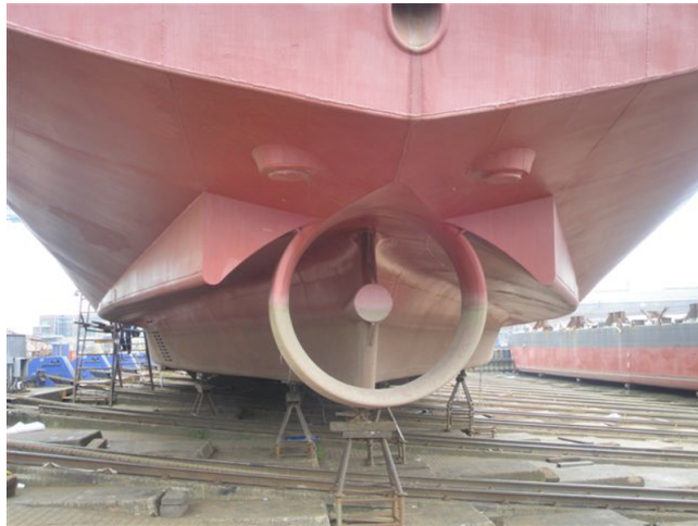
Figure 1.1: Example of an inland ship propeller tunnel. The skirts on the sides are closing off the volume in front of the propeller, so that air is prevented from entering the propeller from upstream. When the propeller is active, its suction will eventually have the tunnel filled with water, so that the propeller can provide sufficient thrust, even when it is only partially submerged in still conditions.
