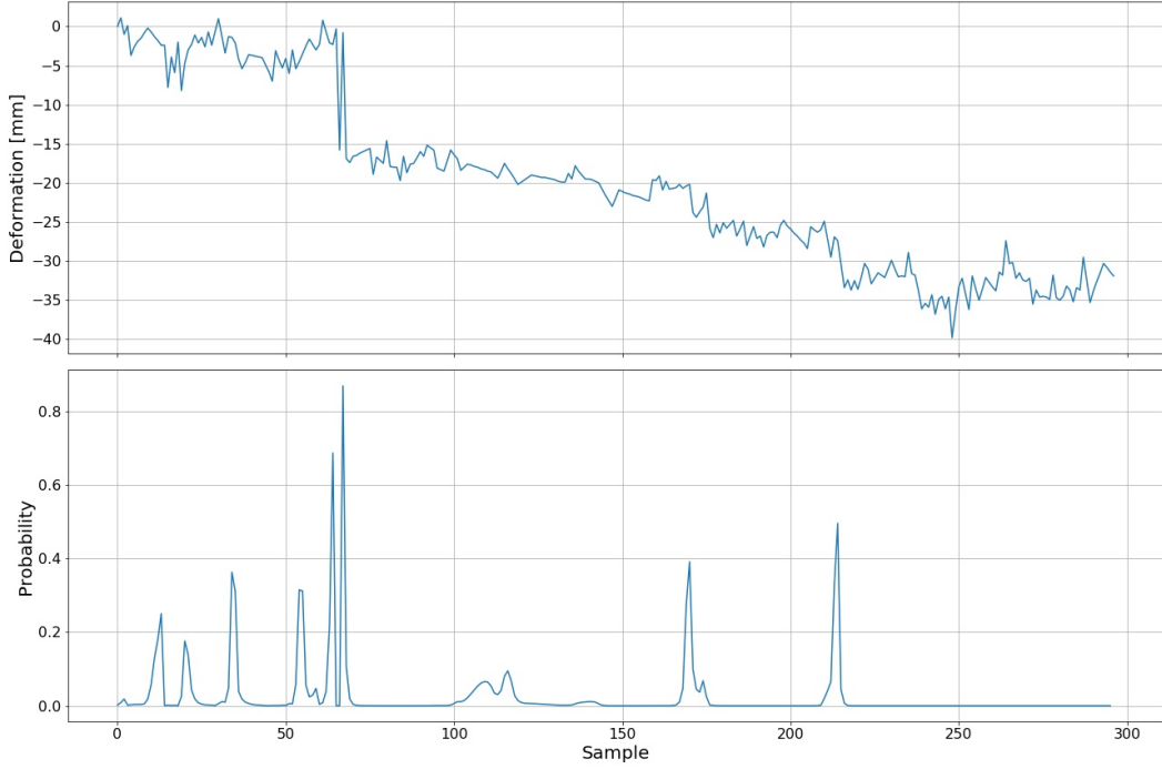
Figure 5-5: An example of the Bayesian Changepoint Detection algorithm outcome for a univariate time-series. A time-series from AL dataset with linear interpolation (top) and the probability score (bottom), AL869. The samples where the probability is higher than 0.3 are treated as changepoints.
