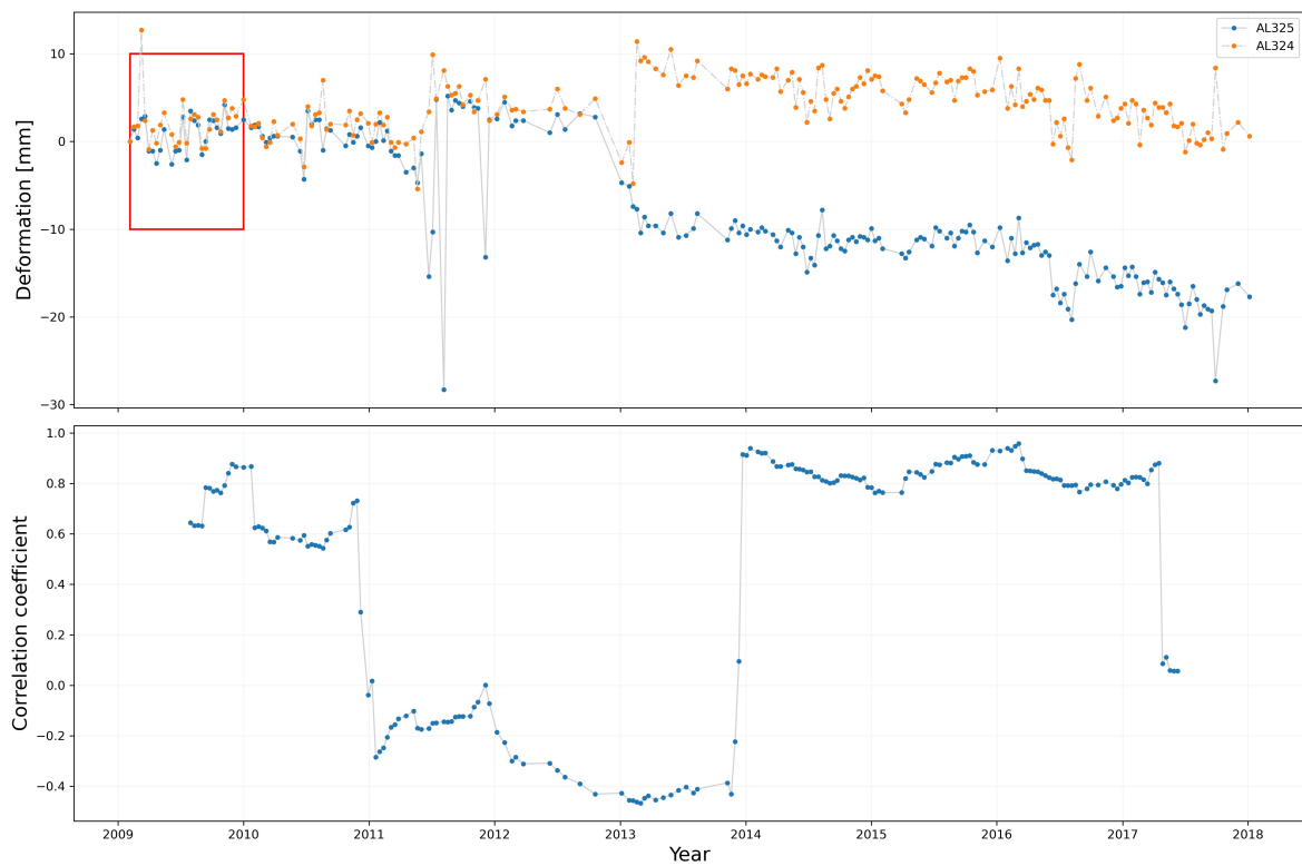
Figure 3-13: Two neighboring time-series AL324 and AL325 (top) and the correlation coefficient calculated with a sliding window of the size 30 (bottom). The window is shown in the top figure in red. The calculated coefficient within the window is centered, i.e. the result is shifted to the center of the window. The correlation coefficient median is 0.7797.
