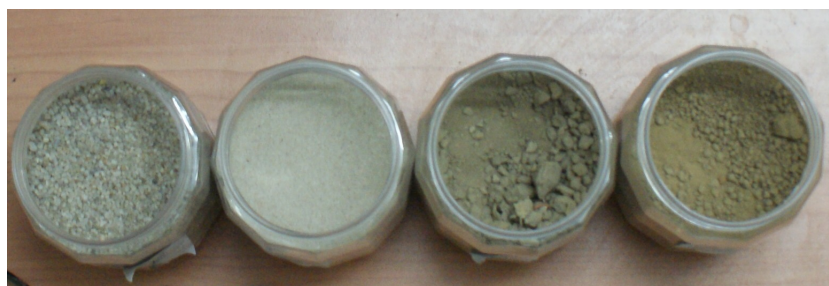
Figure 2. The four different soils used the study. From left to right: Soil 1: Grade I Sand [46], Soil 2: Grade III Sand [46], Soil 3: Silty-loam soil from local field, Soil 4: Graded Silty-loam soil.
