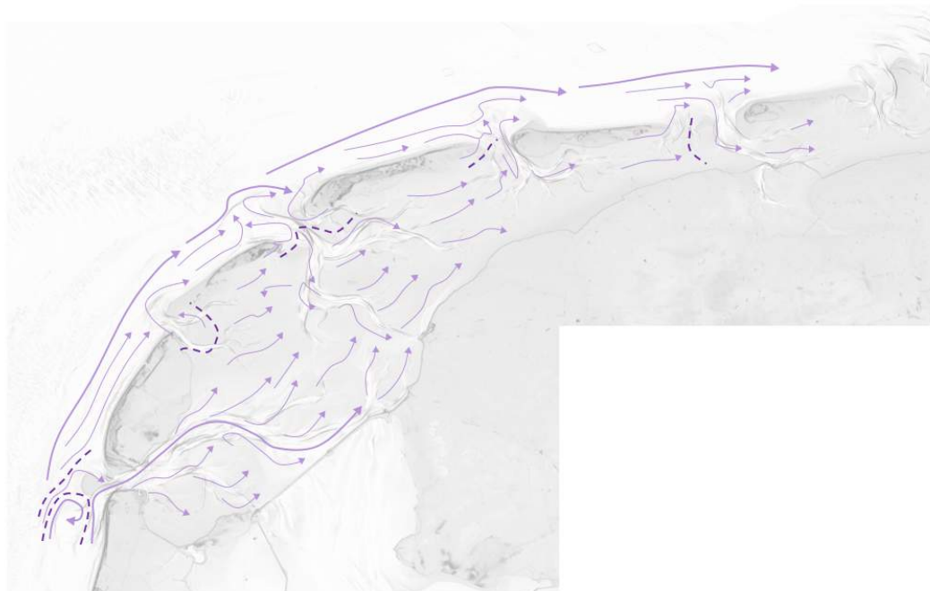
Figure 5.13: Conceptual model of the sediment transport pathways forced by the hydraulic tide, representative wind condition and representative wave condition. The arrows indicate the dominant transport directions. The coloured, dotted lines indicate the position of diverging net sediment transports.
