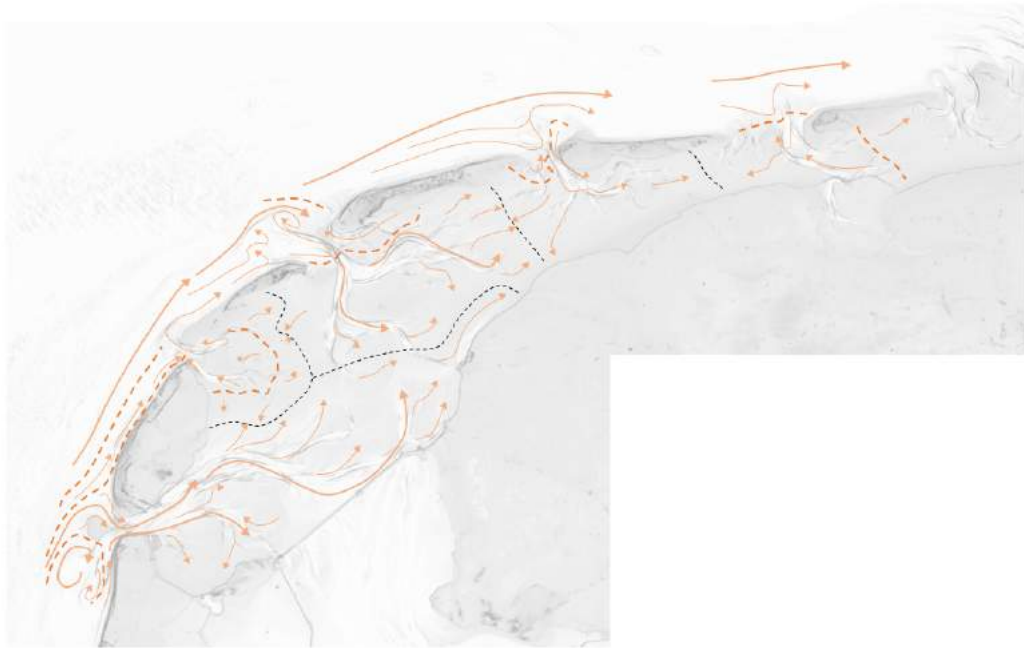
Figure 5.11: Conceptual model of the sediment transport pathways forced by the hydraulic tide. The arrows indicate the dominant transport directions. The coloured, dotted lines indicate the position of diverging net sediment transports. The black, dotted lines indicate the position of the tidal watersheds that do not have net sediment transport over them.
