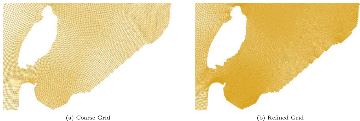
Figure 3.5: The coarse grid configuration and refined grid configuration. Both figures show the grid for the Marsdiep basin. The white blocks in the figures indicate the Noord-Holland coast and Texel.
