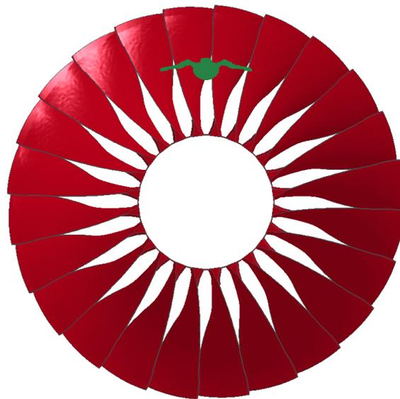
**Figure 4.** The selected impact position and bird orientation.
