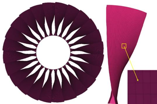
**Figure 3.** Finite element model of turbofan engine fan.
