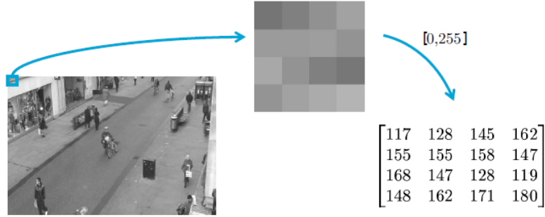
Figure 2-1: This figure shows the transition from a frame of a video to an 8-bit integer valued matrix [1, 12].
