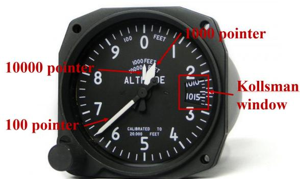
**Figure 3.1:** "Three pointer" altimeter <sup>1</sup>
