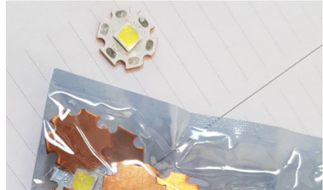
Figure 5.9 _ Cree XHP70, 30W extra high power led, 7x7mm
