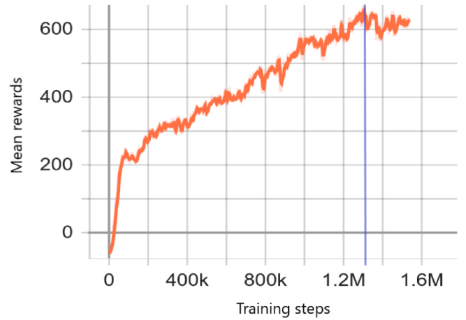
Figure 5: The training phase performance of the PPO model showing the mean rewards per optimization vs training steps. The selected model is indicated by the blue line.
