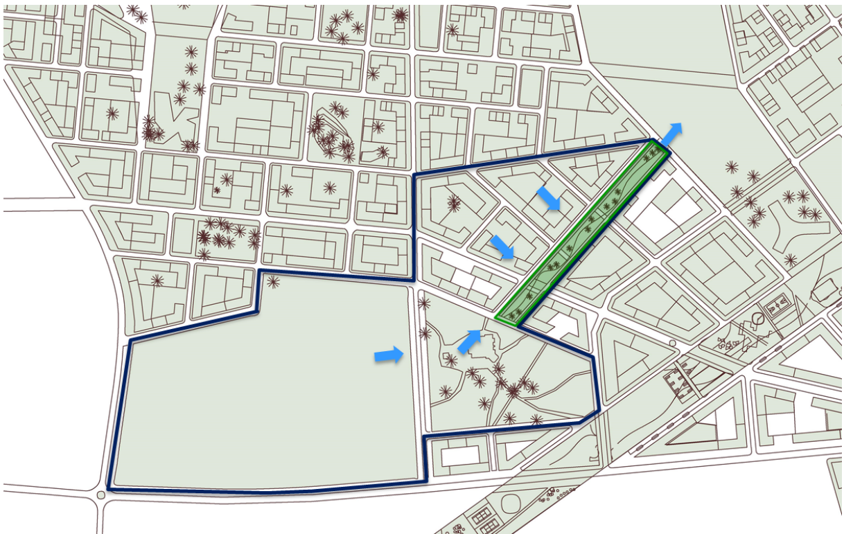
Figure 2: Catchment area (blue polygon) assumed to drain into and discharge via the pilot, respectively.
