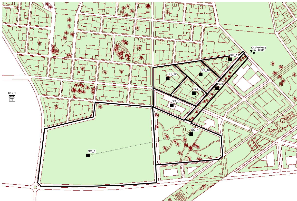
Figure 4: Discretization of the catchment area into subcatchments and their hydrologic connection for modelling with EPA SWMM.
