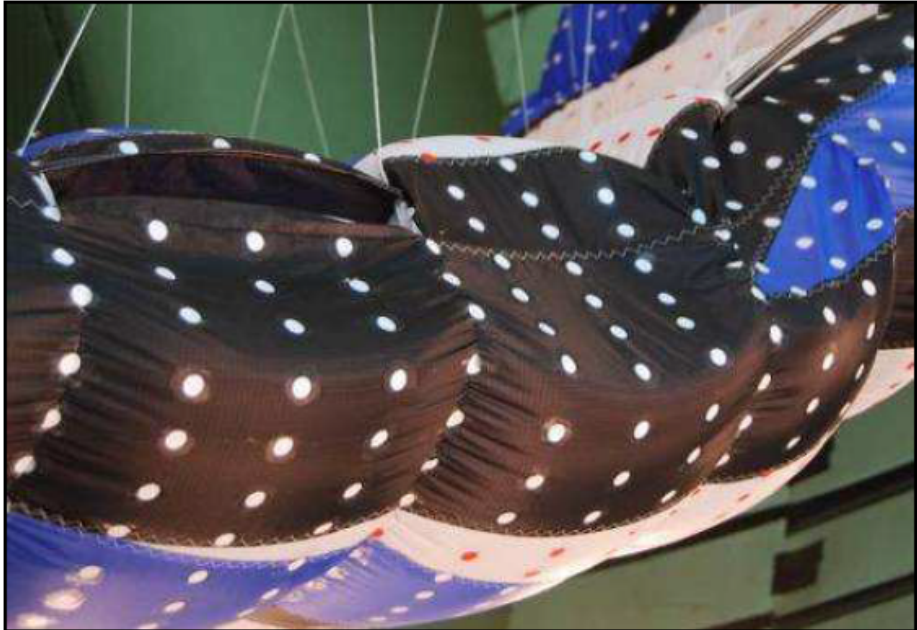
Figure 2.9: Ram-air kite in a wind tunnel experiment by de Wachter [23]. The white dots were used to compute the deformed shape of the parafoil for a CFD analysis. A striking detail are the dents located at the leading edge where the stagnation pressure compresses the membrane structure and the profile loses its curvature.
