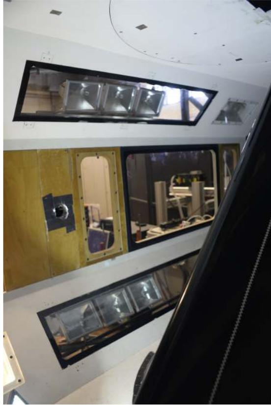
**Figure 3.6:** Illumination system for the infrared thermography experiment. View from inside the wind tunnel.
