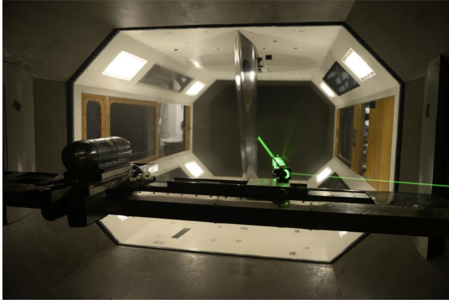
**Figure 3.10:** PIV laser sheet pointing at the investigation volume
