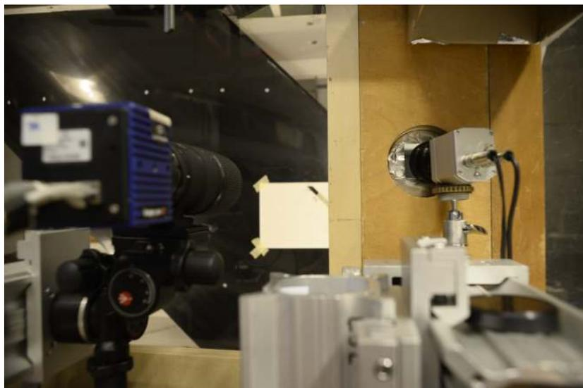
**Figure 3.9:** Close-up of the PIV setup: double camera arrangement for the
