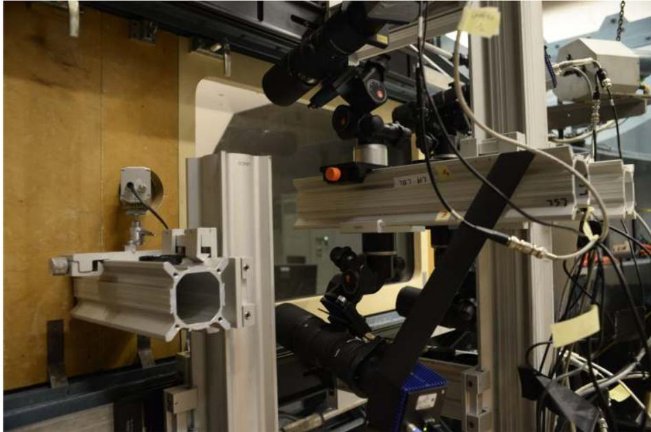
**Figure A.1:** Tomographic PIV setup, inclusive of the thermographic camera
