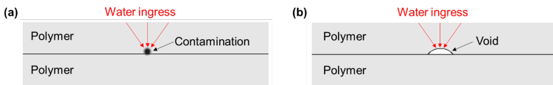
Fig. 2.9. Water ingress mechanisms: (a) contamination or (b) void formation due to loss of adhesion happening at the polymer-polymer interface.
