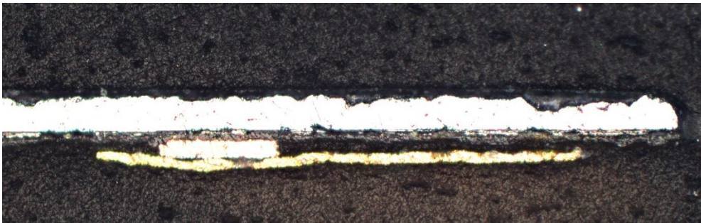
Fig. C.2. Cross-section image of the bump of the RFID chip connected to the gold track using TPU as adhesive – no contact achieved (735 g.).
