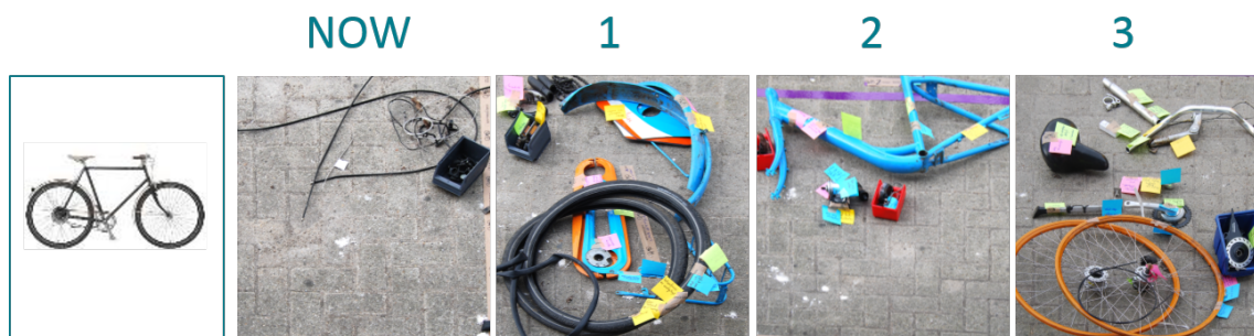
Figure 6: Part Planning Tool. Impression of which parts can potentially be used more than one design generation. Showing respectively parts that cannot be reused (only usable ‘now’), and parts that can be reused or ‘carried over’ up to the first (1), second (2) and third (3) generation of bicycles
