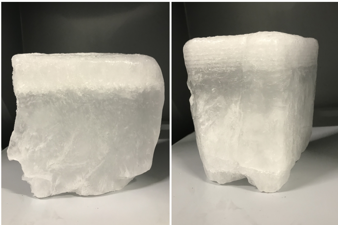
(a) The ice after instant flooding, showing one thick layer (b) The ice after incremental flooding, showing multiple thin layers
