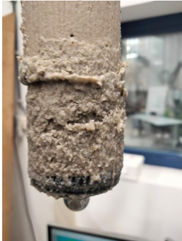
(b) A picture of the drill grout column after it was pulled out of the sample. A build up of sand particles can be seen at the bottom part of the column.
