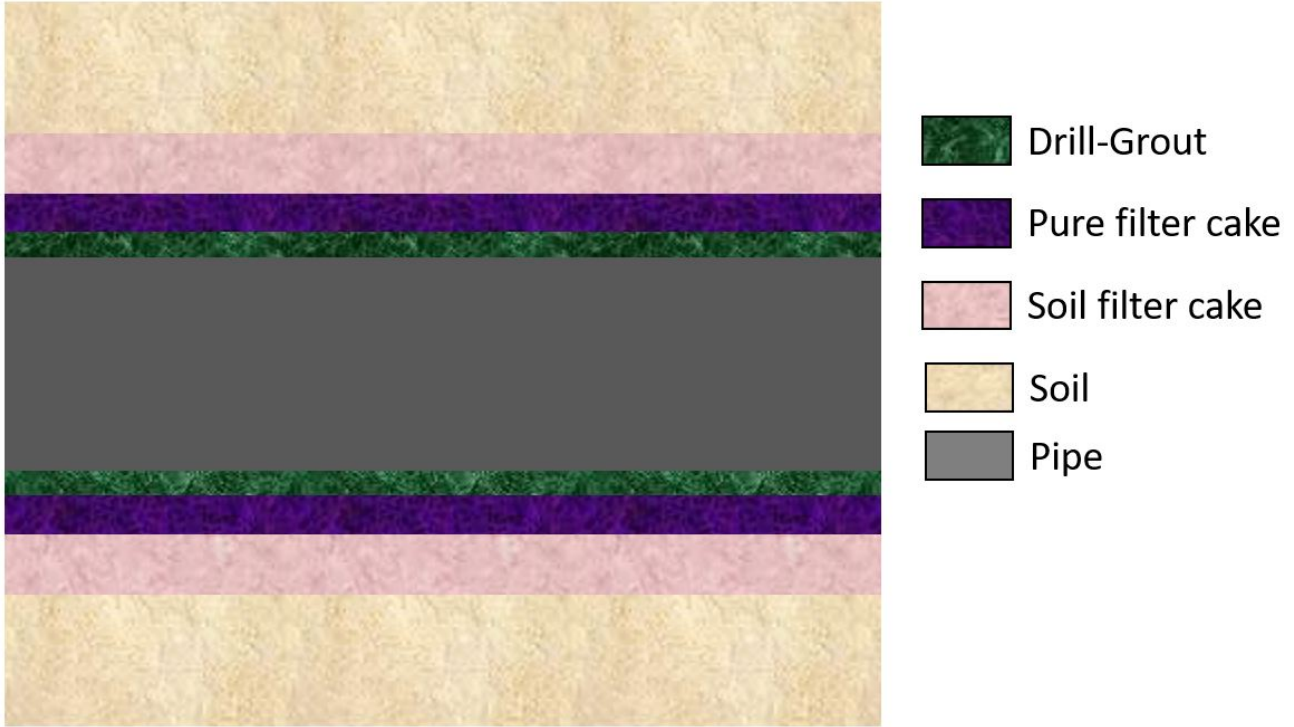
Figure 14: crossection of a borehole filled with drill-grout.
