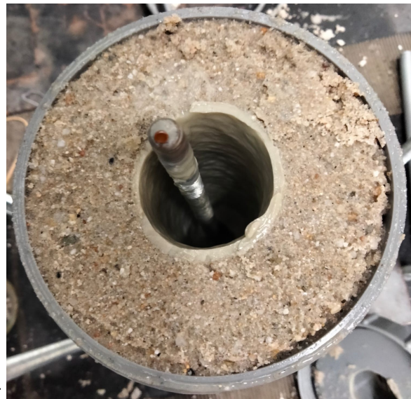
(b) Cross section of a sample where a filter cake has been formed by pressurising drilling fluid, but no drill-grout has been cast afterwards. This was the sample used for test 3.
