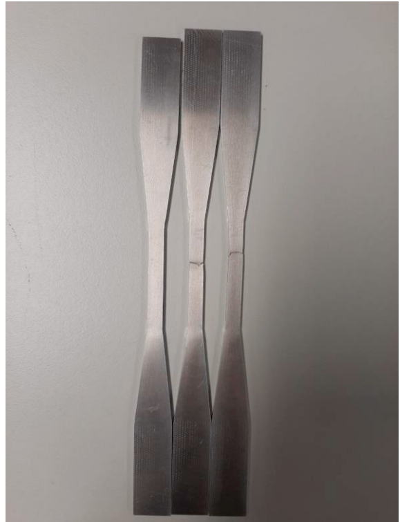
Fig. 4. Yield test structure a) applying tension to a dog-bone aluminum using Instron machine and attached LVDT to measure the strain. B) Comparing two broken specimens with a true specimen
