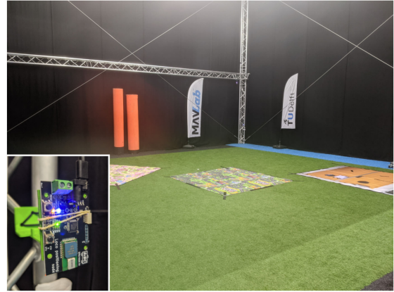
Fig. 2. Flight data was collected in the ‘‘Cyberzoo’’ at TU Delft using a Crazyflie drone and the loco positioning system by bitcraze. Groundtruth is provided by an Optitrack motion capture system.
