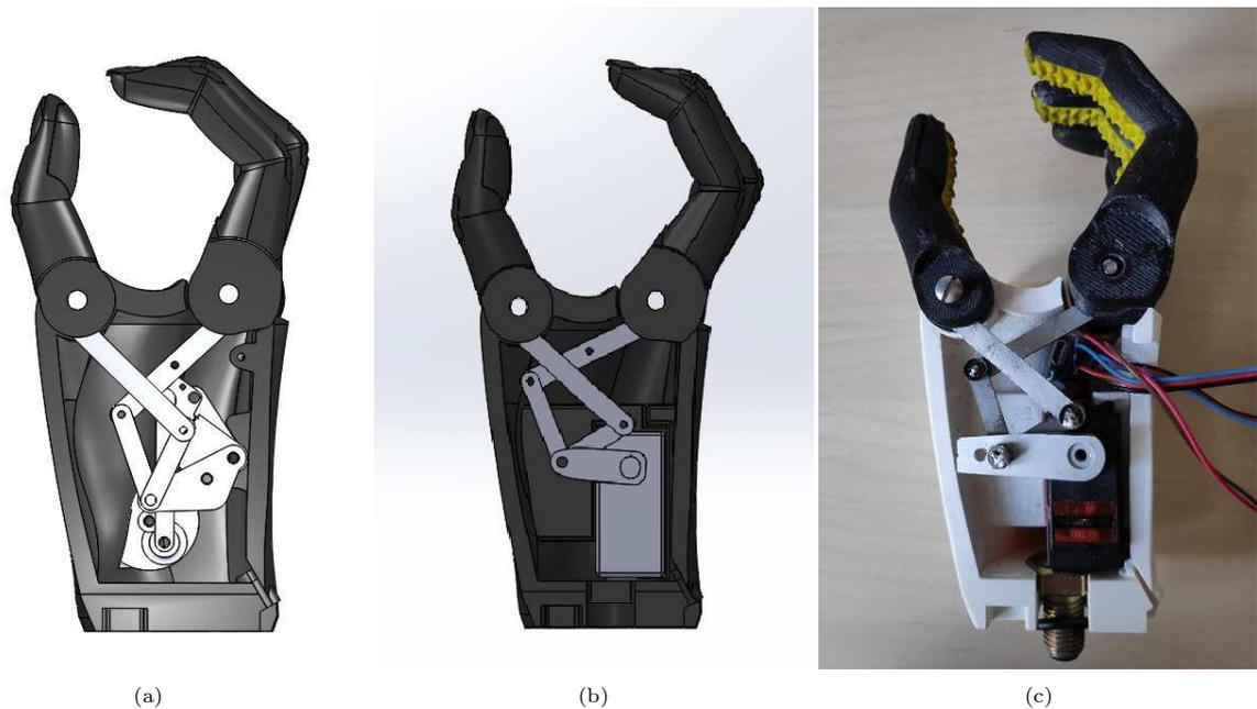
Figure 4.1: (a) The original 100 dollar hand. (b) The revised 100 dollar hand, (c) Realization of the prototype.
