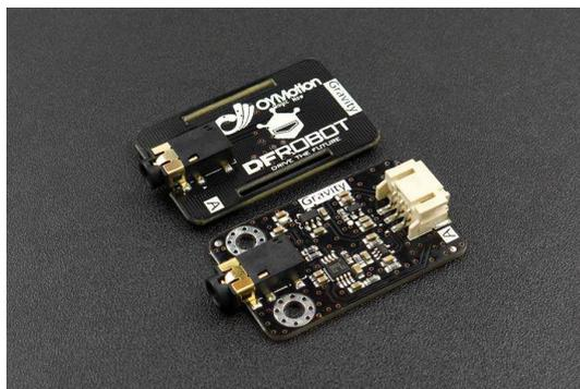
Figure 4.2: The DFRobot EMG sensor by Oymotion.
